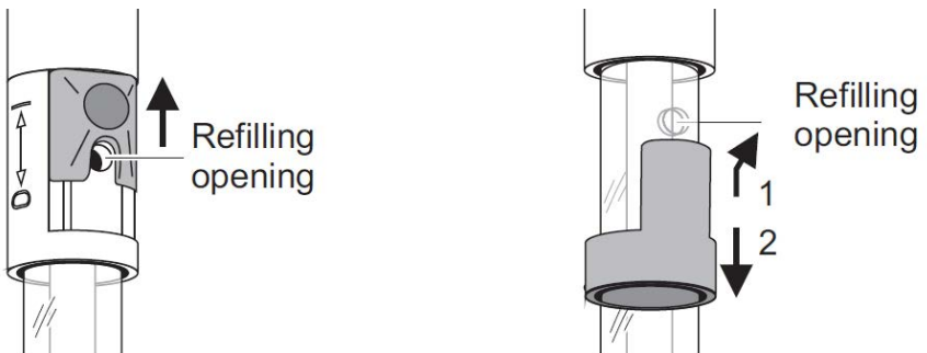
Figure 3.4: Slider (left) and stopper (right) refill openings for YSI lab electrodes
