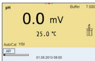
Figure 3.6: mV display on the YSI MultiLab during pH calibration
