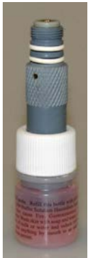
Figure 4.2: Long term storage of field pH electrode
