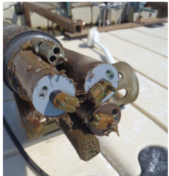
YSI 6600V2-4 with antifouling components after 30-day deployment in Tampa Bay, FL, USA
