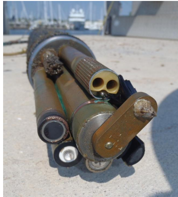
EXO2 sonde with central wiping brush and other antifouling components after 30-day deployment in Tampa Bay, FL, USA
